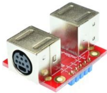
Figure 3: mDIN7-F-F-V1A with headers
